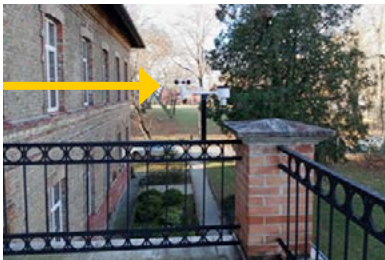
Weather station installed at the balcony of Lánczos Kornél Gimnázium about 6 meters from the ground floor, on a pole welded to the railing
